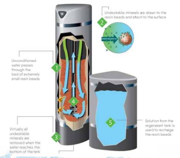
The conditionedwater passes up through the filter tube and is distributed throughout the house
